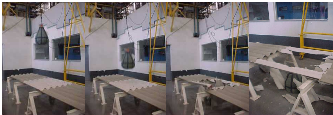
Figure 8 – Impact resistance test (600 J) of asbestos corrugated sheet P7 – 6mm.
