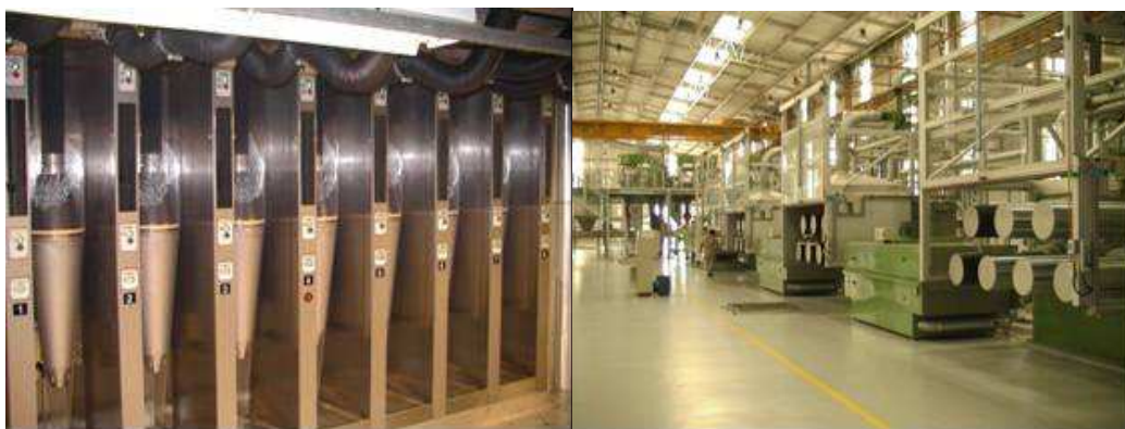
Figure 1 – Spinning and drawing processes for producing PP Brasifil
