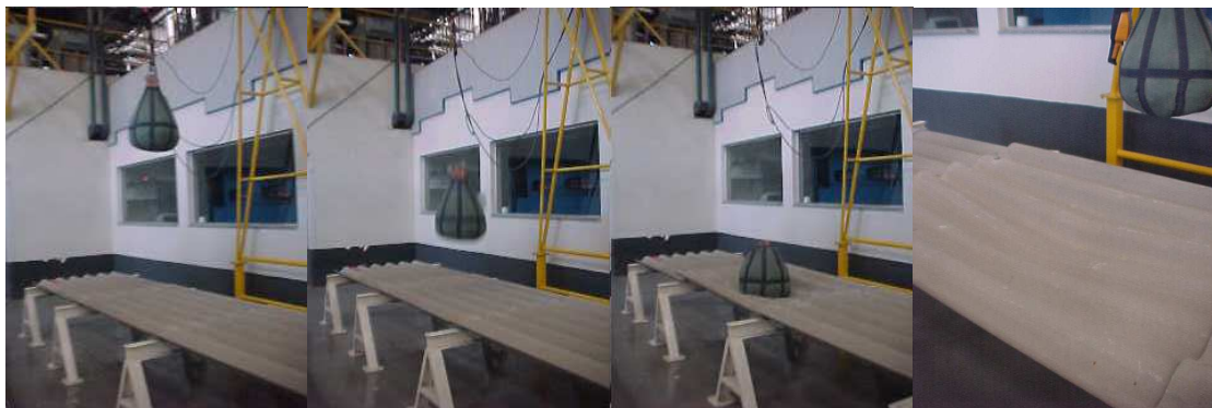
Figure 7 – Impact resistance test (600 J) of corrugated sheet P7 – 6 mm using Brasifil.
